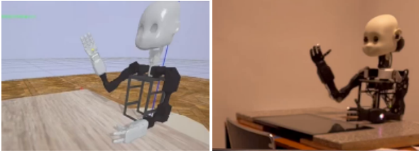
Fig. 2: Simulated NICO in myGym environment (left), and its physical counterpart (right).
